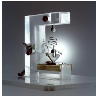
Figure 1.3 - Point contact transistor. Adapted from ref. 10
