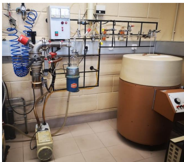
Figure 3.16 - Photograph of the vacuum drop-microcalorimeter apparatus.
