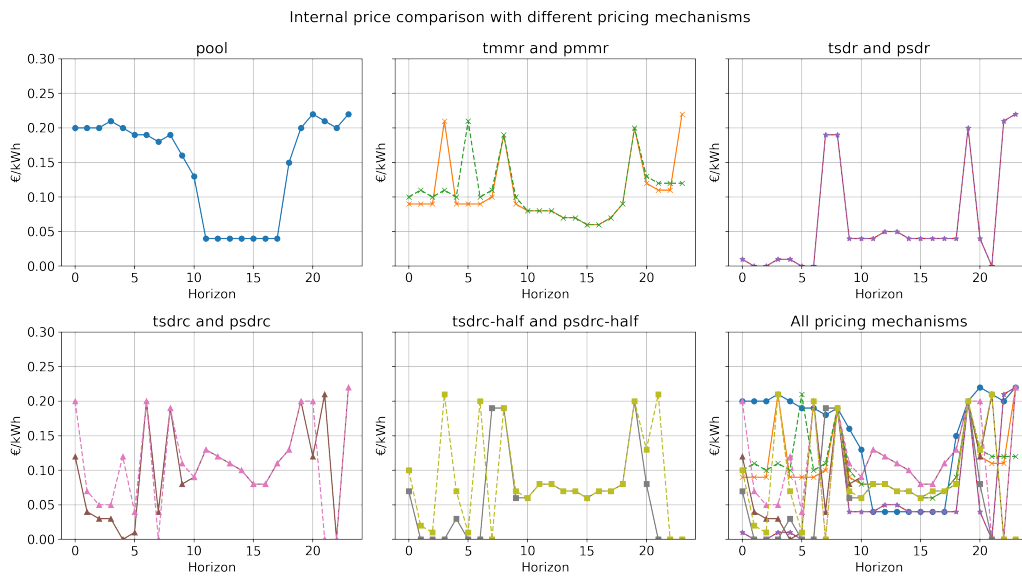
Figure 4.48: LEM internal prices per pricing mechanism, Total and Partial comparison in Scenario 4
