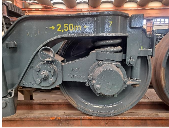
Figure 17 - Primary suspension and Axle guide of ARCO passenger cars, taken in CP workshop in Guifões.
