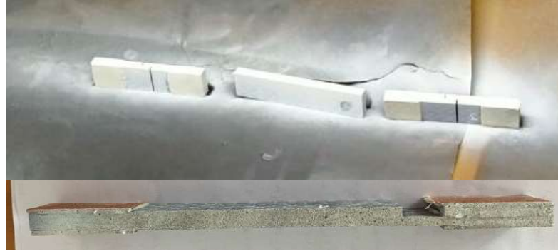
Figure 29 – Specimens preparation: Application of white paint in TAST specimens, then the speckle pattern in a CLS specimen.
