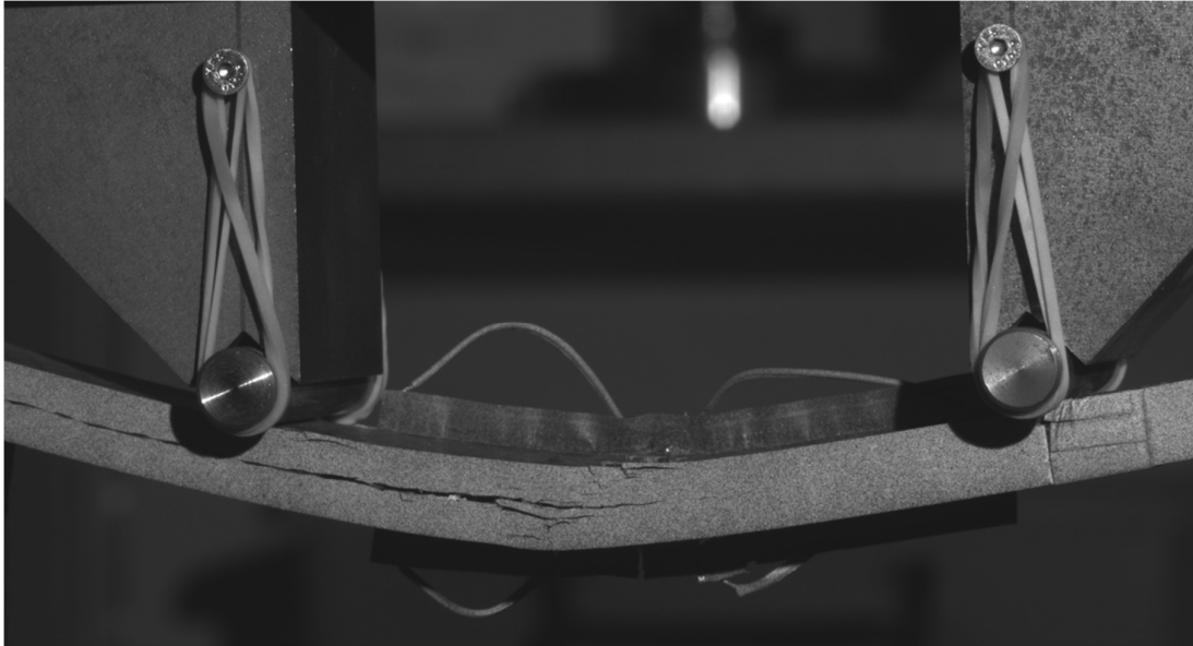
Figure 37 – Long 4ENF DIC image at 100% of the duration of the test (end of the test).
