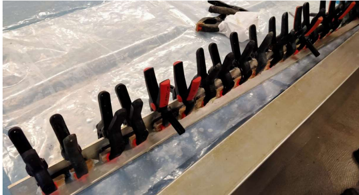
Figure 28 – TAST specimens adhesive drying after the application of the bonded tabs.
