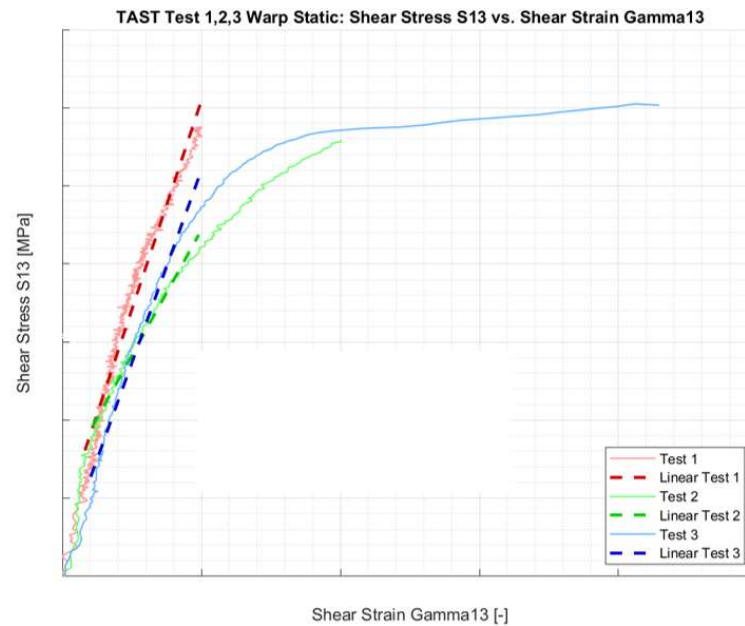
Graph 7 – TAST warp direction tests with individual linear slope curves: Shear Stress vs Strain.
