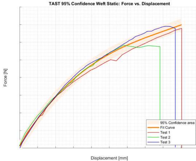
Graph 10 – TAST weft direction tests with 95% confidence region: Load vs Displacement.
