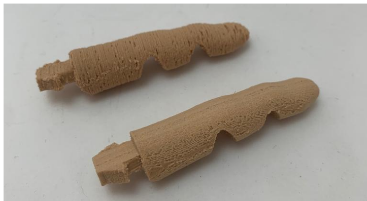
Figure 68 - Comparison between parts printed in different directions.
