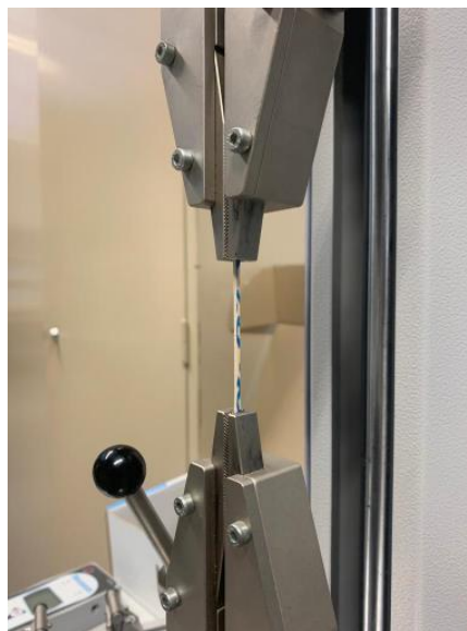
Figure 30 - Tensile tests made to the different formulations.
