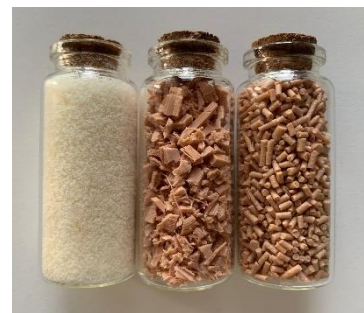
Figure 3: PU, TPU and pellets from the mixture
