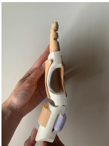
Figure 75 - Representation of the mechanical movement of the Flexygrip.
