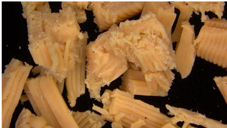
Figure 24 - TPU waste - under microscope analysis.
