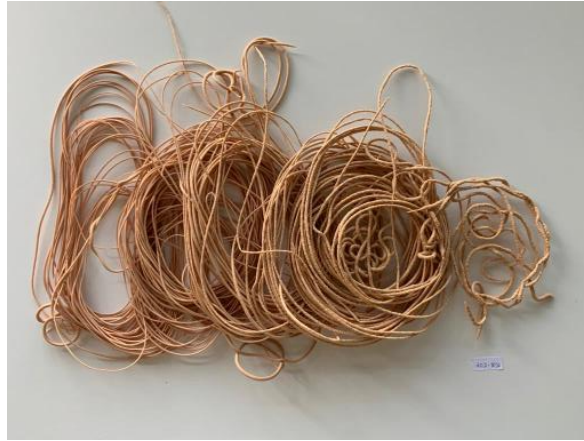
Figure 37 - Filament extruded before going through grinding into pellets (20 % PU + 80 % TPU).
