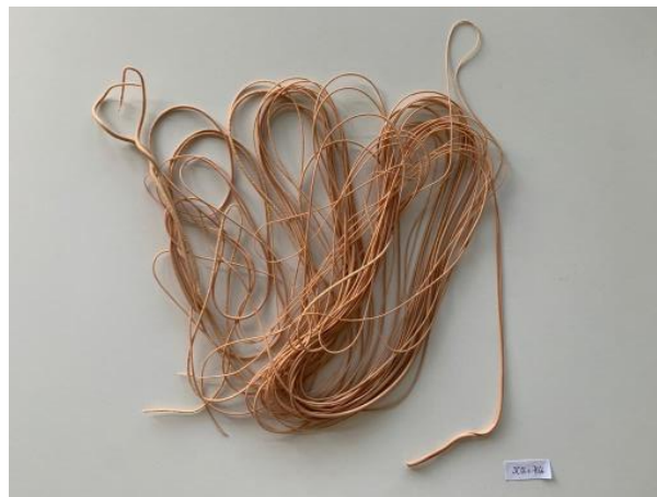
Figure 38 - Filament extruded before going through grinding into pellets (30 % PU + 70 % TPU).
