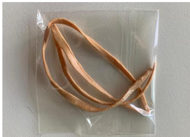
Figure 52 - Flattened filament example with the developed material.
