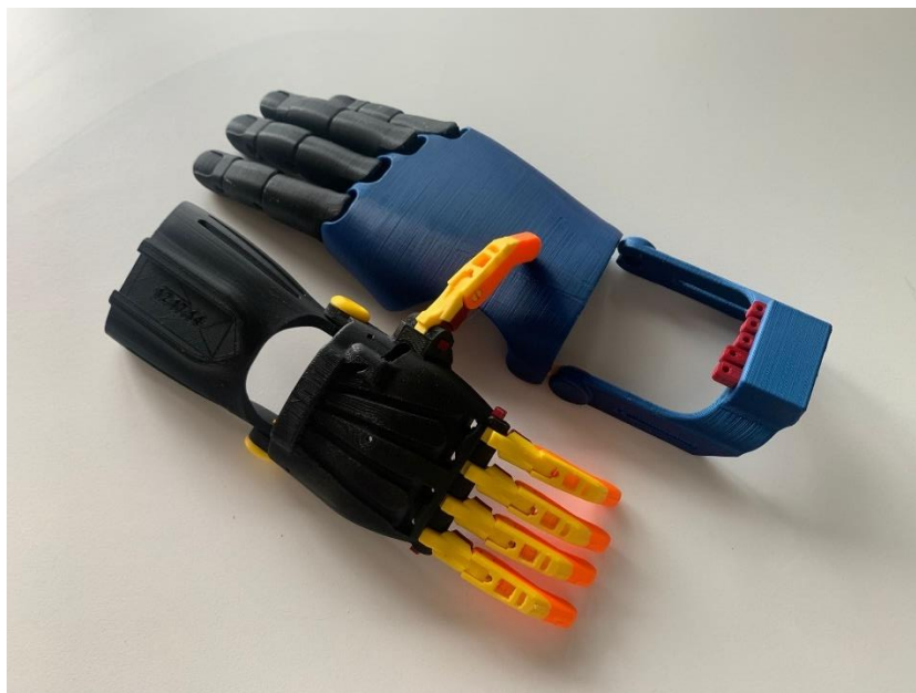
Figure 63 - E-Nable standart hands 3D printed for study of the assembly and mechanical properties.
