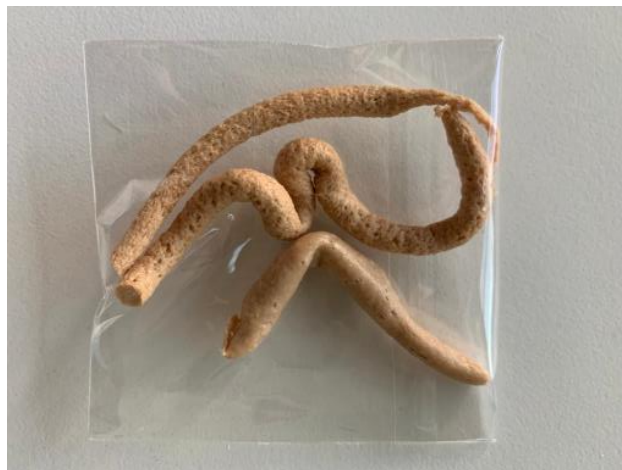
Figure 48 - Melt fracture example with the developed material.
