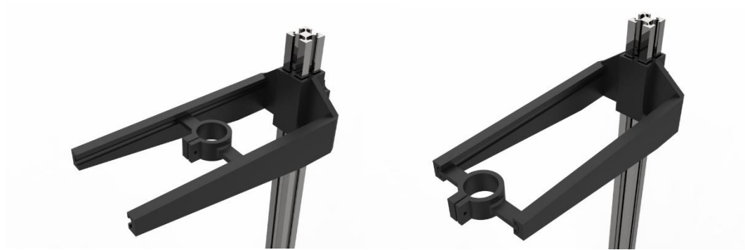
Figure 2 - Render of the movement of the head of the drilling support for PU blocks.
