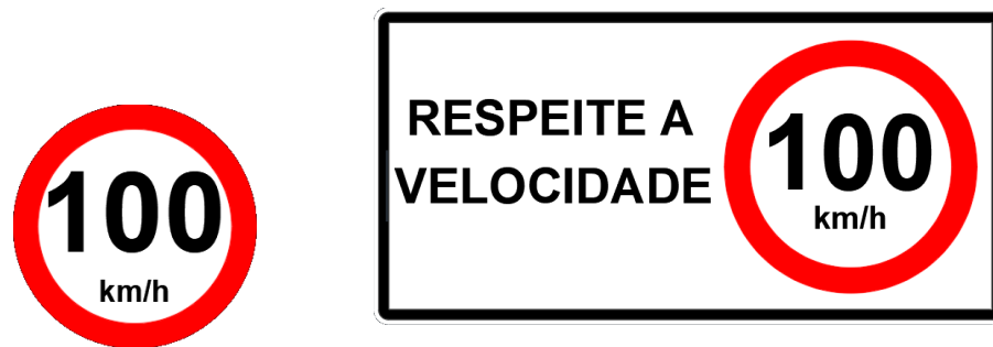
Figure 7.7: “Regular” speed limit sign (left) and speed limit sign placed before the peripheral line countermeasures (right) depicting the “regard the speed” message
