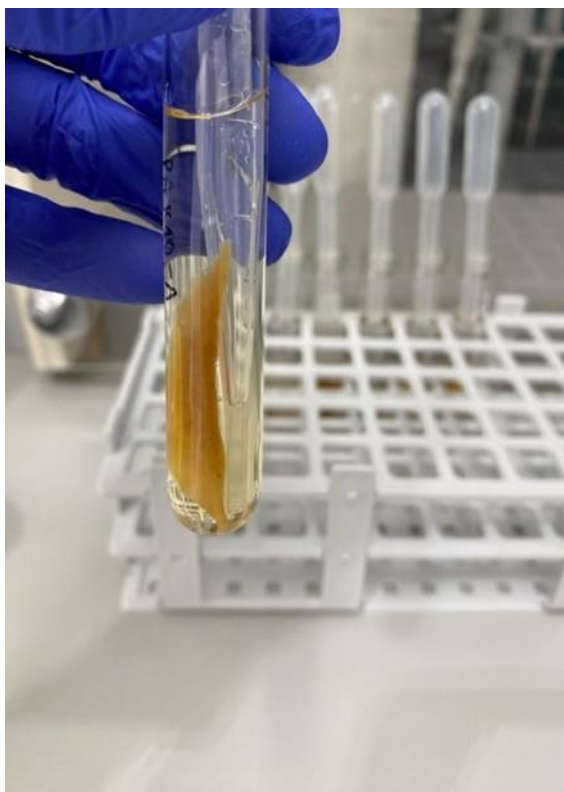
Figure 7 Example of test tube with bone cut soaked in HCl (0.5 M).
