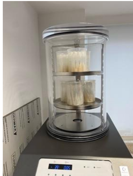
Figure 10 Samples placed in the freeze-dryer (HyperCOOL HC3055).
