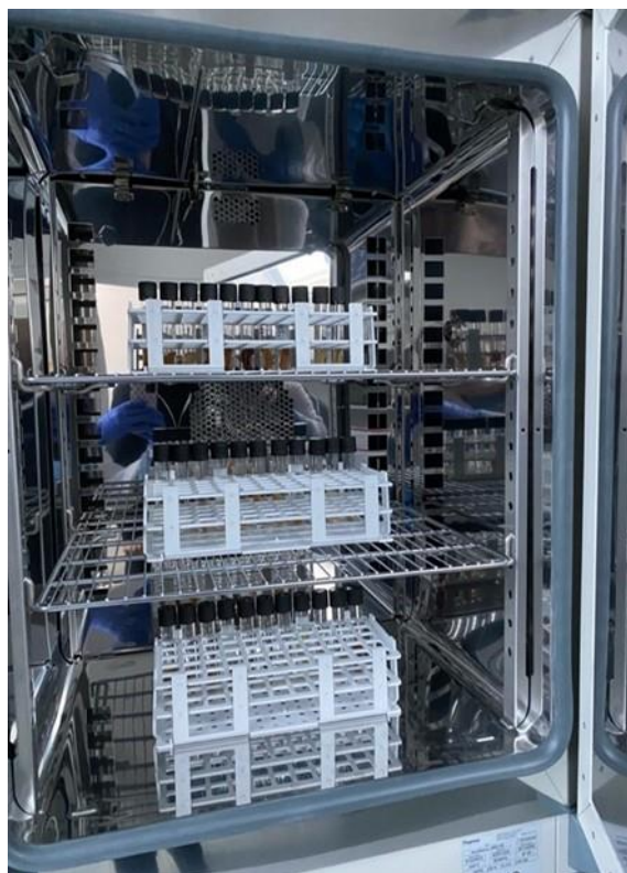
Figure 8 Samples placed in the oven (Thermo Scientific™ dry sterilizer)
