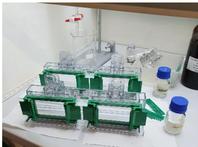
Figure 3.3 - Representation of a typical setup when gels were being prepared. The flasks contain the separating (closer to the camera) and the stacking gel solutions. In the figure, the separating gel is polymerizing inside the assembly.
