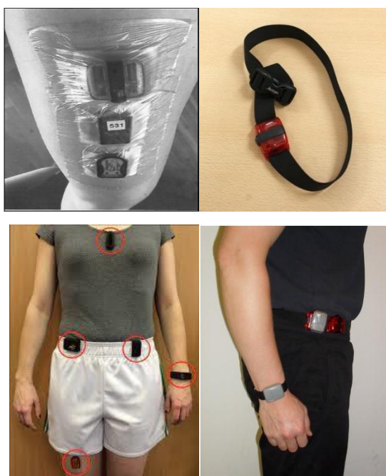
Figure 4: various types of accelerometers and the possibilities of locations
