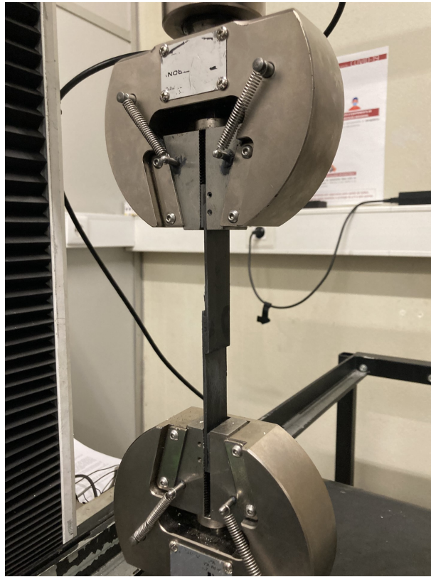
Figure 4.10: Mounted CFRP SLJ with 50 [mm] overlap
