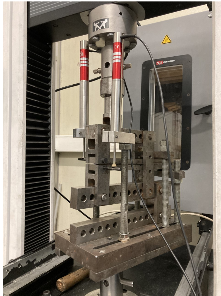
Figure 4.9: Mixed-mode apparatus setup [56]
