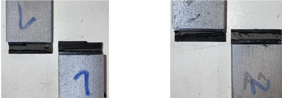
Figure 12: Failure mode for two TAST specimens
