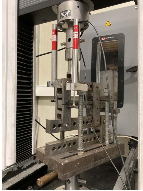
Figure 7: Apparatus for mixed-mode [13]
