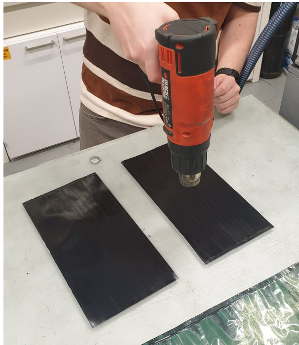
Figure 3.18: Heat application in the final stage of the sheets layup
