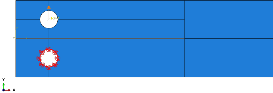
Figure 13: Boundary conditions for the DCB specimen model
