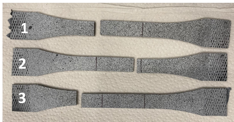
Figure 4.2: Bulk specimen failure modes
