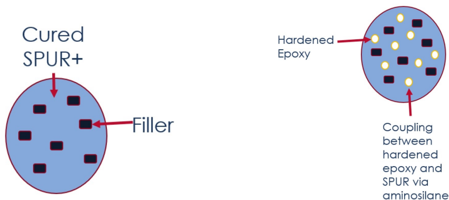
Figure 3.1: Provided representation of the precipitates in the cured SPUR without (at the left) and with the epoxy resin part B (at the right). Adapted from Momentive Performance Materials Inc. ®
