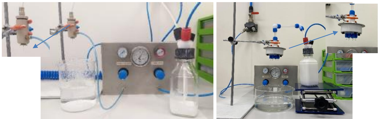
Figure 9- Spheres' production method. A) nanoXIM•G1000 granules' encapsulator; B) nanoXIM•G2000 granules' encapsulator.
