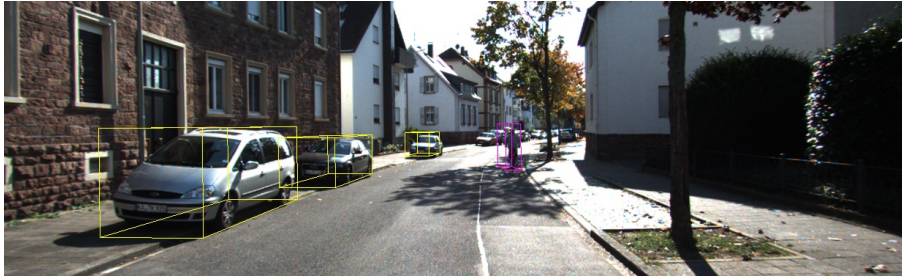
Figure 4.2: Example of 3D detection of PointPillars using Vitis AI Library samples.
