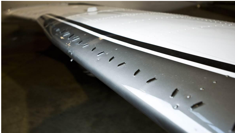
Figure 2.4: Vortex generators in an aircraft wing [24].
