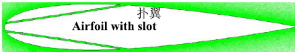
Figure 2.6: Leading-edge slots at the upper and bottom surfaces [27].
