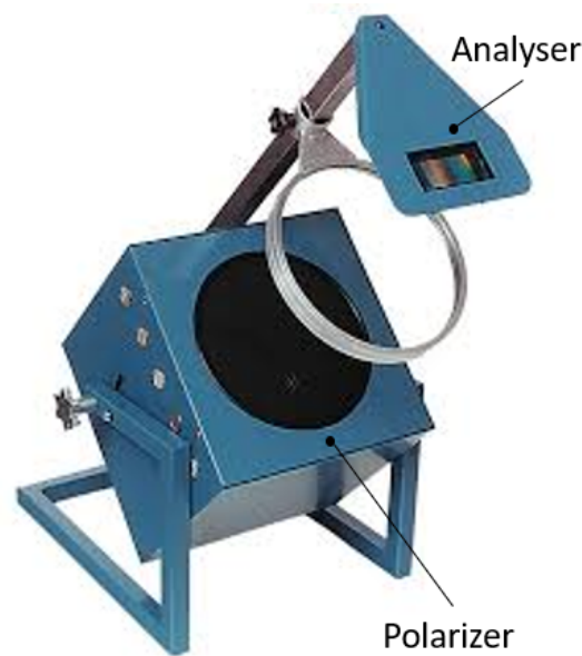
Figure 2.4: Polariscope with polarizer and analyser filters, adapted from BA Glass (2023).
