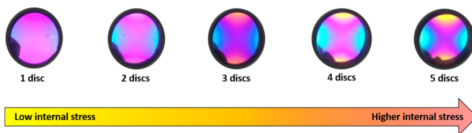
Figure 2.5: Set of strain disks of a polariscope, adapted from BA Glass (2023).
