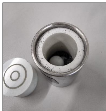
Figure 11 – Ball milling vessel ready to go to the mixer mill with zirconia balls and reactants inside.
