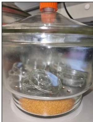
Figure 15 – Samples in a vacuum desiccator after hydrolysis reaction.
