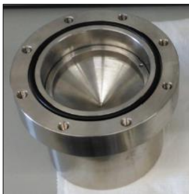
Figure 9 – Open cross-section of MRc with an o-ring placed.
