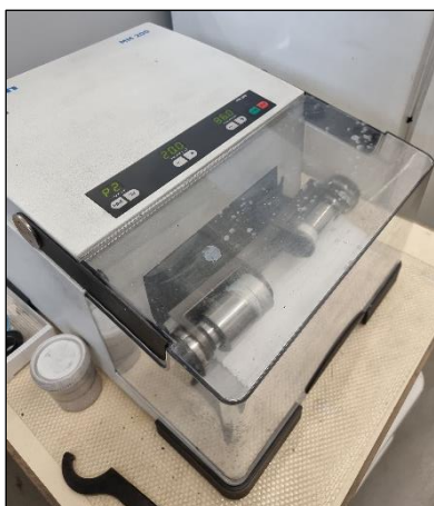
Figure 10 – RETSCH MM200 mixer mill with 2 ball milling vessels.
