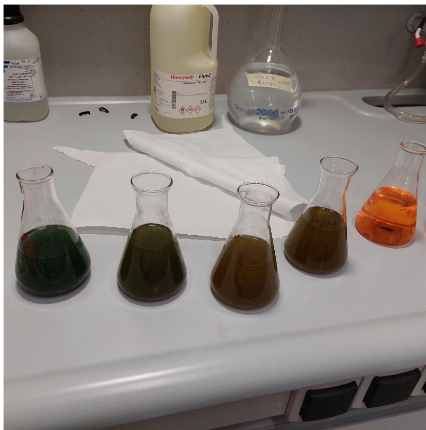
Figure 10 – Determination of total organic carbon. Samples after addition of K_2Cr_2O_7 and before titration
