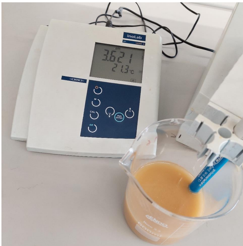
Figure 8 – NAG pH measurement before titration, using WTW InoLab pH Level 1 pH Meter
