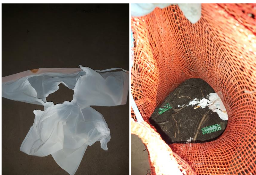
Figure 3.7. Sample of torn bioplastic B bag (left) and bioplastic B bag and corresponding strips inside a burlap bag (right).
