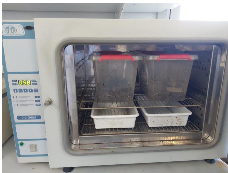
Figure 3.5. Experimental set-up for simulated industrial composting trials.
