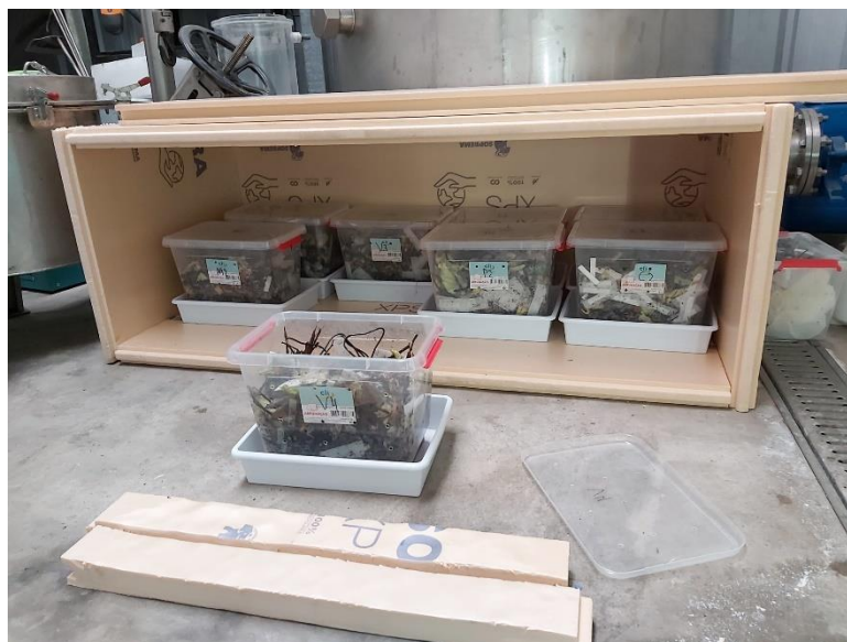
Figure 3.6. Experimental set-up for simulated home composting trials.
