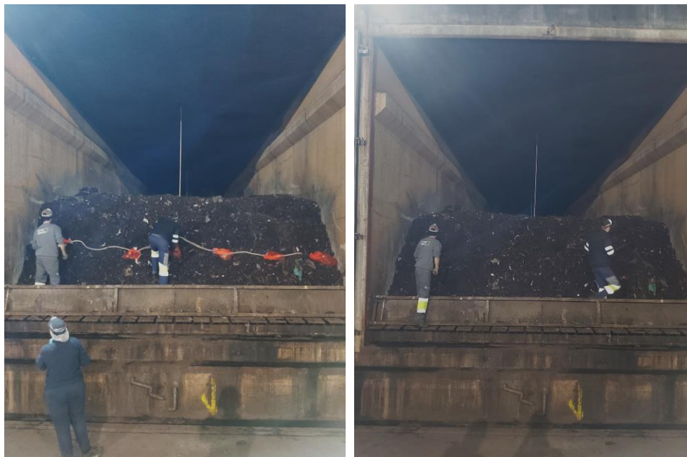
Figure 3.8. Arrangement of the samples in the composting tunnel before covering (left) and after covering (right).
