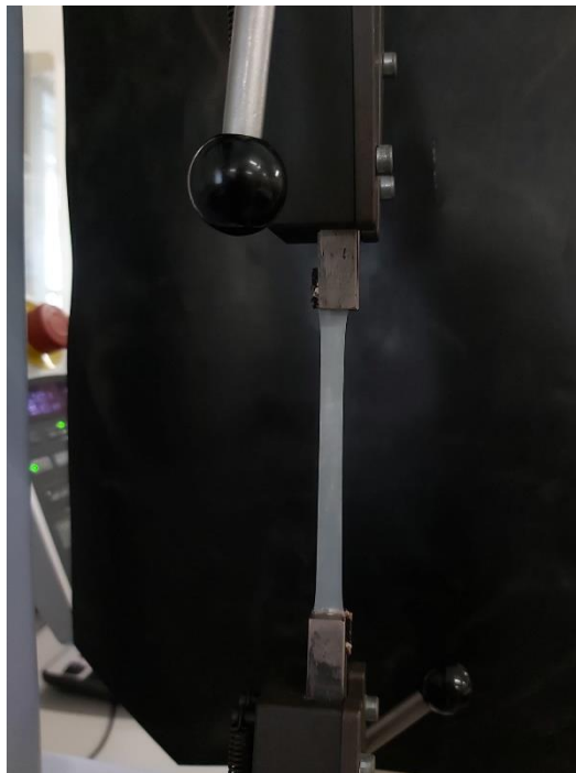
Figure 4.8. Example of a tensile test for a strip of BA (Bioplastic A).
