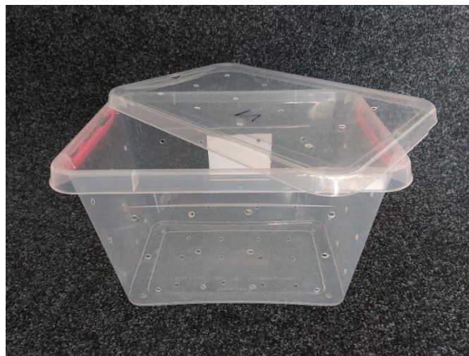
Figure 3.2. Photographic record of the plastic boxes used to contain the biodegradable material during composting in the laboratory trials.
