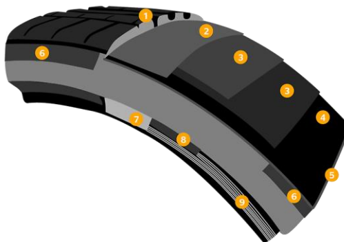
Figure 2. Passenger car tire design [11].
