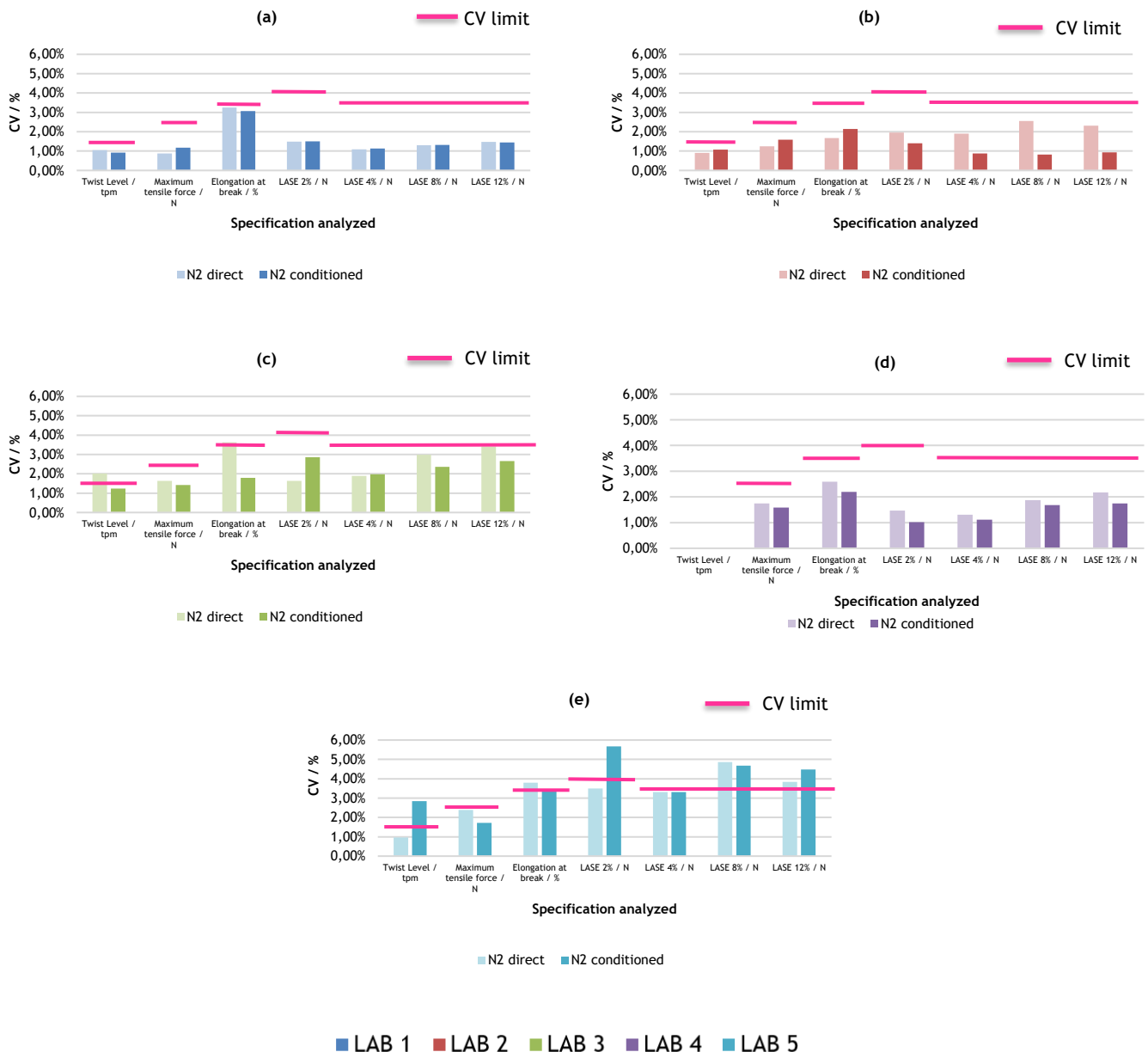
Figure 32. Coefficient of variation of N2 for each laboratory (direct and conditioned testing).
