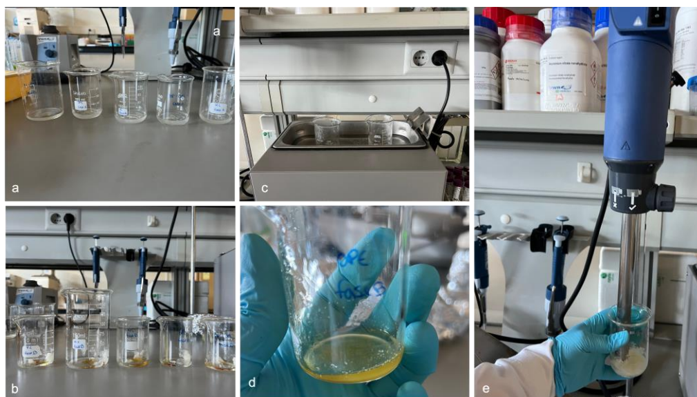
Figure E.0.1 - Sunscreen production steps: a- goblets containing phase A; b - Goblets containing phase B; c - Phase A and Phase B in heating bath until dissolution; d – Dissolved phase B; e - Homogenization until the production of a homogenized emulsion.
