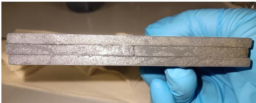
Figure 4.12 Film from test 1 applied in the PVC substrate, covering the cut executed in the middle plate.
