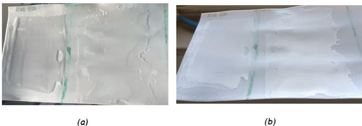
Figure 4.1 Film ID6: (a) right after application in the polished (left) and non-polished (right) gasket; and (b) after drying in the polished (left) and non-polished (right) gasket.
