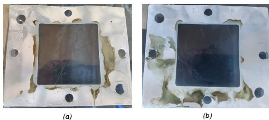
Figure A.3 Photos of the gaskets covered with 500 µm of ID7 film, dried at 40 °C, after experiment with gasket 2 - (a) is one of the gaskets and (b) is the other one.
