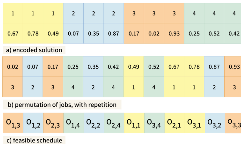
Figure 3.5. Decoding a chromosome into a list of ordered operations.
