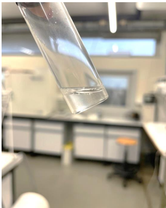
Fig. A1.1. Example of a cloud point.
