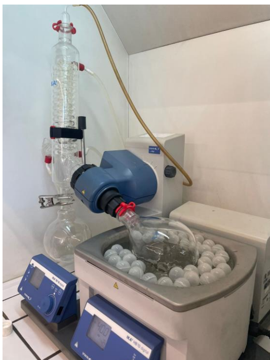
Fig. C1.2. Drying of the ionic liquid by reduced-pressure distillation, at 323.15 K, in a rotary evaporator.
