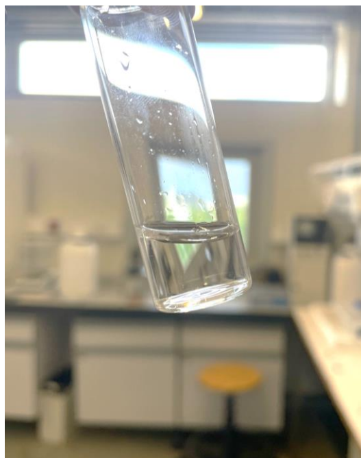
Fig. A1.2. Example of a clear mixture, not in cloud point.
