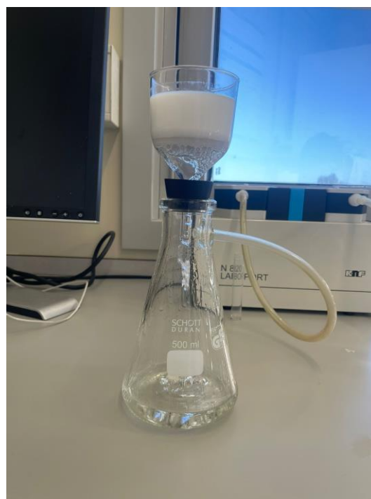
Fig. C1.3. Drying of the ionic liquid by reduced-pressure filtration.
