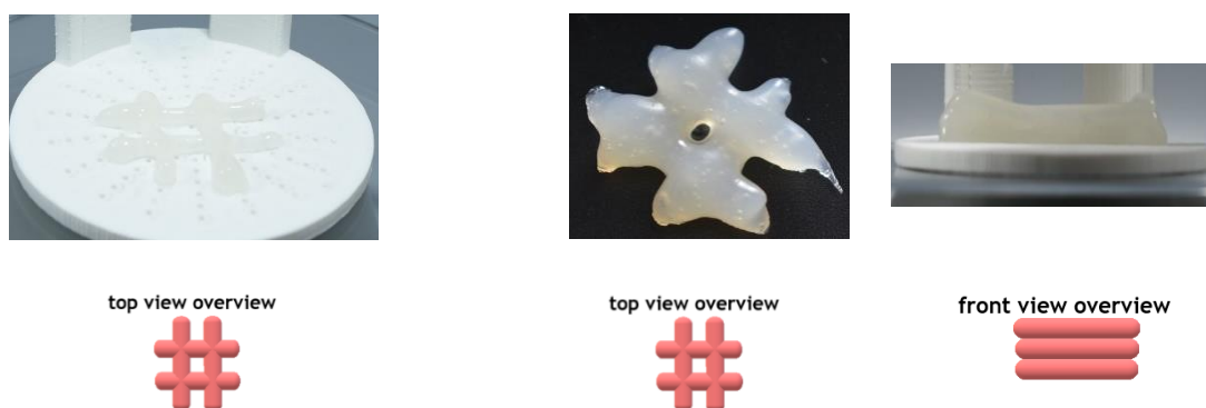
Figure 4.9. Proof of the concept for 2.3:5:92.7 FCL-5T-CNF-2 sample: syringe diameter of 0.686 mm for 2-layer (left side) and syringe diameter of 2 mm for 2 and 3-layer structure (right side)
