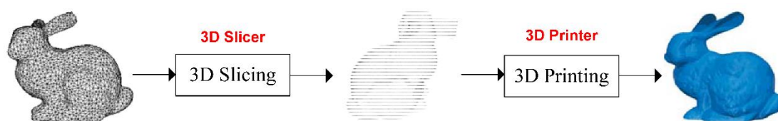
Figure 12 - Process from 3D model to 3D printable model. Adapted from Pham, G. N., Lee, S.-H., Kwon, O.-H. & Kwon, K.-R. A 3D Printing Model Watermarking Algorithm Based on 3D Slicing and Feature Points. Electronics 7 (2018), with permission.
