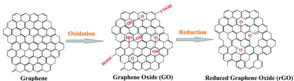
Figure 6 - The crystal structure of graphene, GO and rGO and the process used to obtain GO and rGO from graphene [98].
