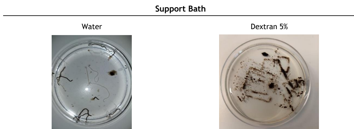
Figure 24 - Printing of the ink into dH 2 O or Dextran 5% at room temperature.
