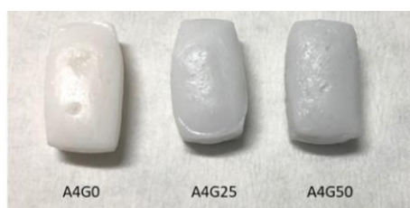
Figure 11 - Macroscopic images of hydrogels with different concentrations of GO (A4G0, A4G25, A4G50). Adapted from [124], with permission from Elsevier.
