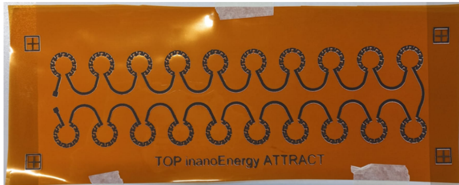
FIGURE 3.19: Screen-printed prototype consisting of 20 radial TEGs connected in series.
