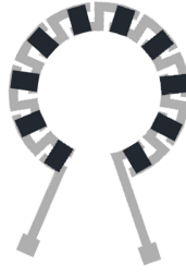
FIGURE 3.1: Schematic illustration of the designed radial TEG composed of thermoelectric stripes (black) and electric contacts (grey).
