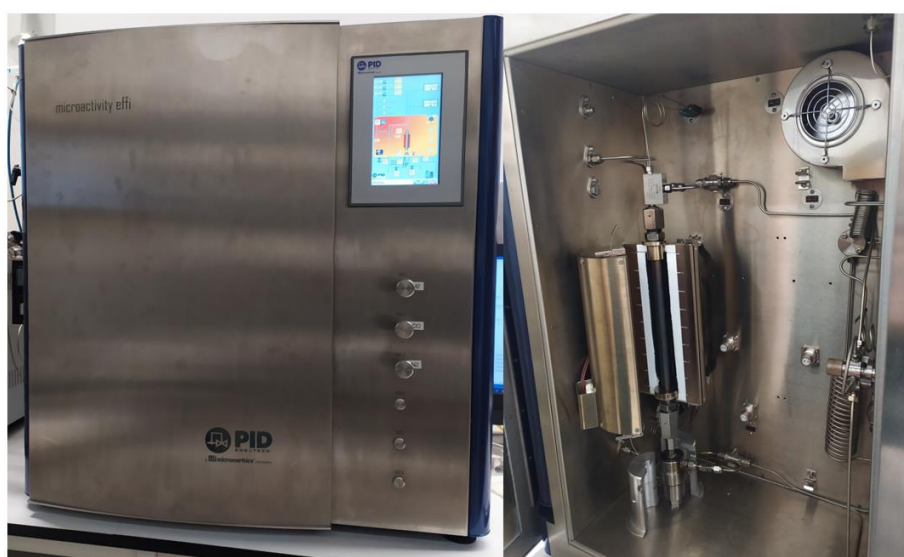
Figure a.9. FTS reactor. External view on the left side and internal on the right.
