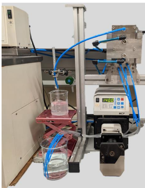
Figure a.2. Image from NETmix configuration for template-free formulations for experiments with different Re_d .
