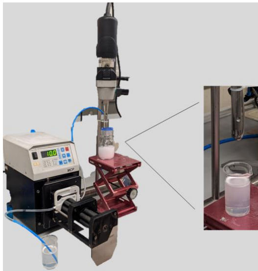
Figure a.1. Experimental configuration used to prepare solution (1) for template-free formulations assays.
