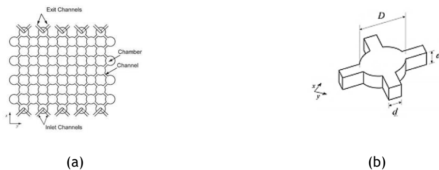
Figure C.1. Schematic representation of a MicroNETmix network, a), and a 2D unit cell, b). Reutilized with permission from Lopes, et al. [54]. Copyright 2023 American Chemical Society.
