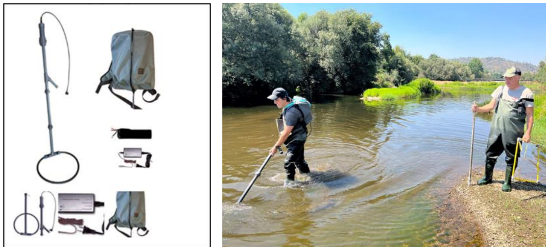
Figure 21 Mobile Reader kit contents (left) and 1 st and 2 nd operators monitoring in the river (right).
