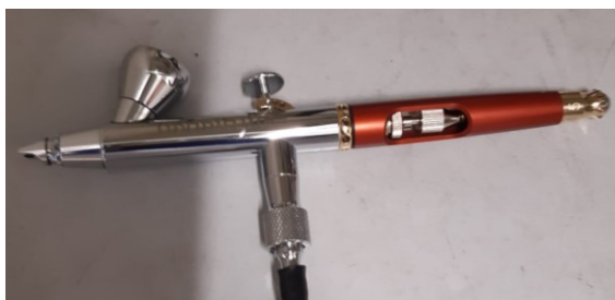
Figure A.2 - Airbrush used for the catalytic depositions.
