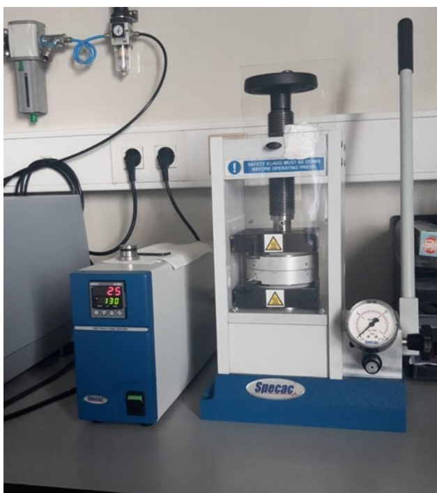
Figure A.5 - Experimental setup for the MEA pressing.
