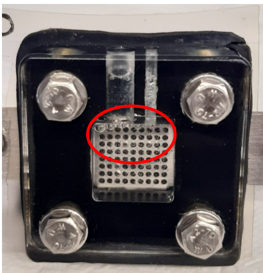
Figure B.49 - Visualization of the CO 2 bubbles at the anode side.
