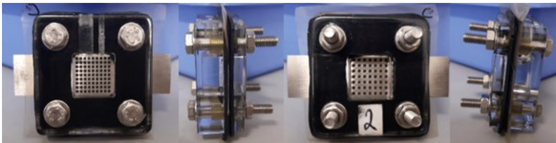
Figure 3.1 - mpDMFC used in the experimental work (front and lateral view, respectively)
