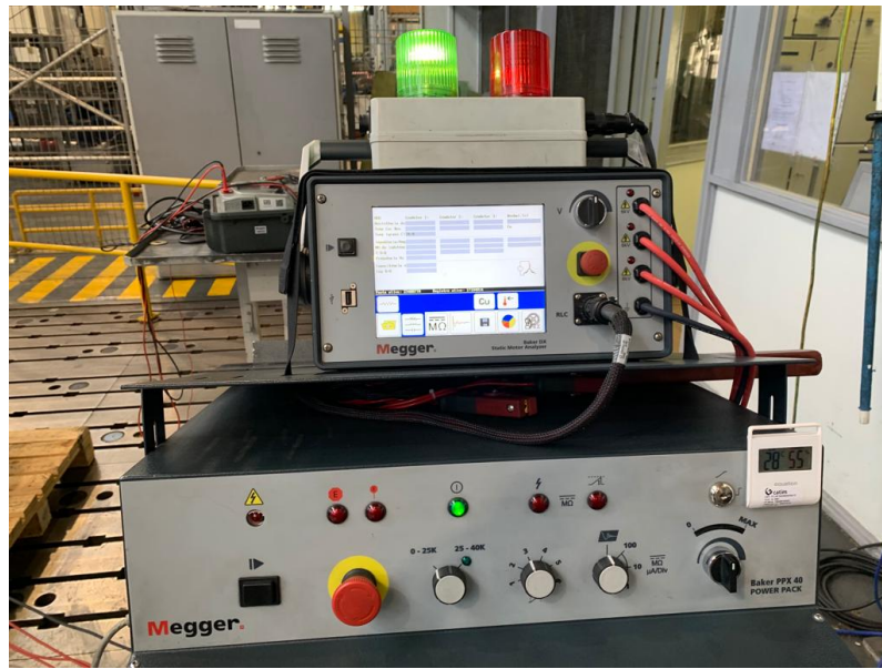
Figure 3.10: Impulse voltage generator Megger Baker DX6
