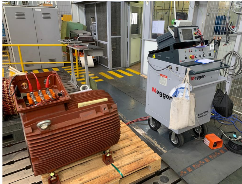
Figure 3.8: Laboratory Setup of the proposed testing system: Test Sample (left) and Megger Baker DX6 (right)
