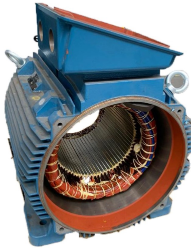
Figure 3.3: Complete winding of a WEG Induction Motor
