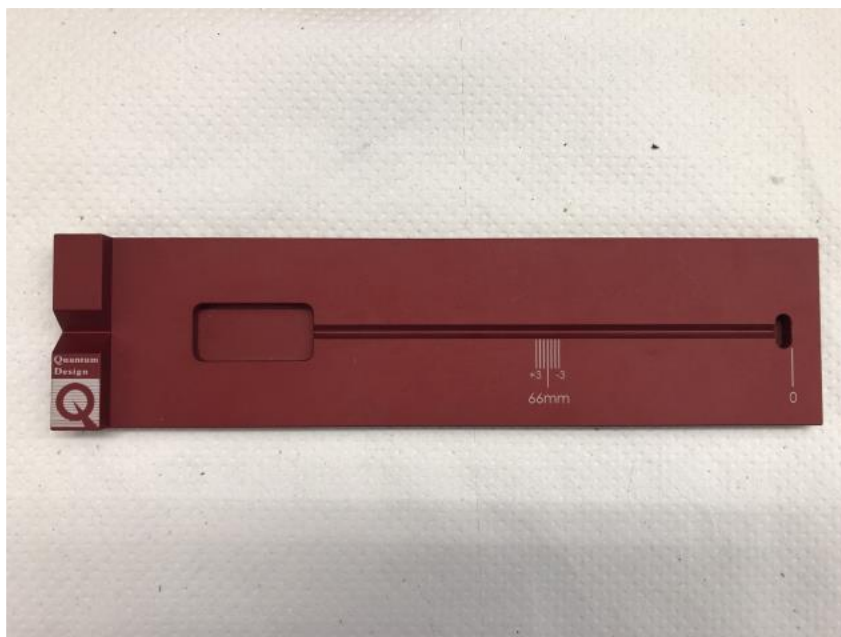
Figure 5.3 - SQUID accessory to place the sample in the right spot.
