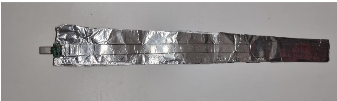
Figure 6.1: INSIGHT™ Sensor covered with aluminium tape
