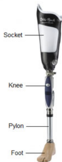
Figure 1.2: Parts of transfemoral prosthesis [4]
