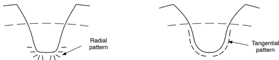
Figure 3.7: Effect of tooth's fillet shape on fiber orientation [39].
