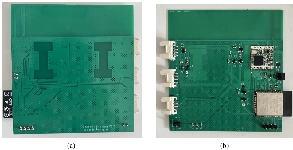
Figure 5.7: (a) Top and (b) bottom sides of the Node1 board.
