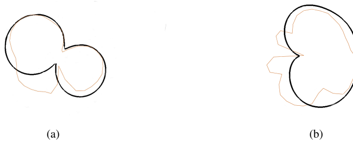
Figure 6.6: Simulated (black) and measured (orange) radiation pattern's shape comparison for the (a) E-Plane and on the (b) H-Plane.
