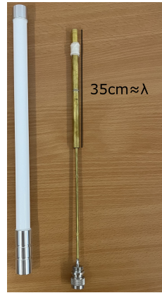
Figure 6.8: 2.15 dBi half-wave sleeve dipole used for the LoRaWAN gateway.
