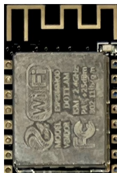
Figure 3.7: 2.4 GHz meandered PIFA (top part of the image) used by an ESP8266 module made by Espressif Systems.
