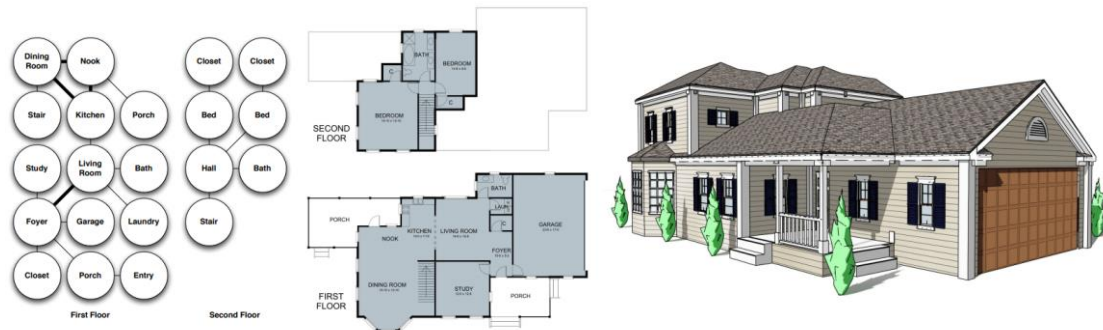
Figure 7 - A bubble diagram (left), generated by a Bayesian network trained on real-world data. A set of generated floor plans (middle). A 3D model (right), generated from the floor plans.
