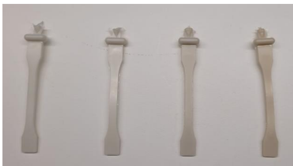
Figure 7. Polymer specimens processed at 140, 160, 175 and 185 °C, respectively.
