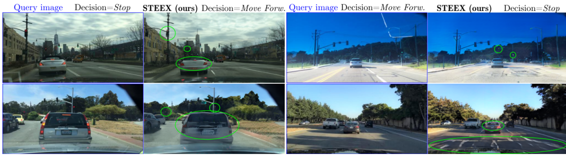
Figure 3.1: Counterfactual explanations generated by the STEEX framework. The regions highlighted contain the modifications made to the original images. In the first image, the decision changed because the car in front starts moving and the traffic light is green, while the second image contains the reverse situation.
