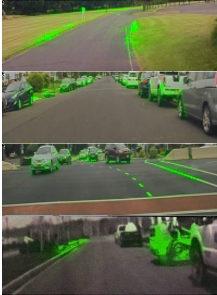
Figure 3.3: Pilotnet [3] saliency maps. The most valuable pixels for the model are highlighted in green. The maps displayed were obtained using VisualBackprop . As expected, the algorithm highlights the lanes and other vehicles on the road.
