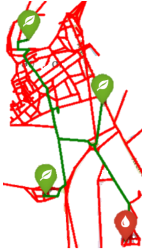
Figure 49 – Schematic representation of the heating pipeline network obtained for simulation 6.
