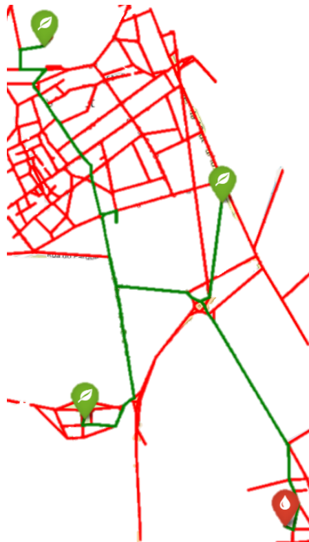
Figure 41 – Schematic representation of the heating pipeline network obtained for simulation 5.
