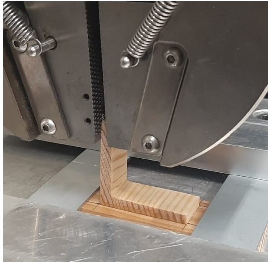
Figure 4: Experimental setup for testing the L-joints.
