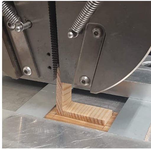
Figure 5.4: Experimental setup for testing the L-joints.
