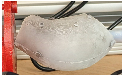
Figure 4.4: Result obtained from painting with the water-based paint.
