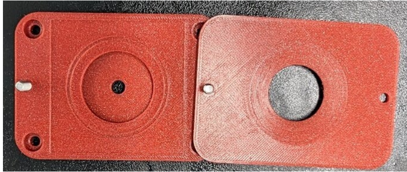
Figure 6.1: Mechanism used to secure the sample for the experimental procedure.
