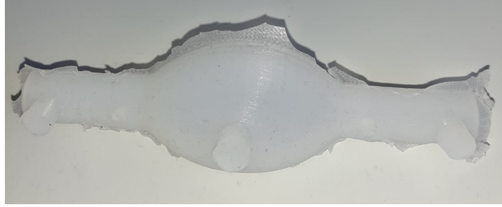
Figure 3.4: First iteration of the balloon after using the BVOH filament.
