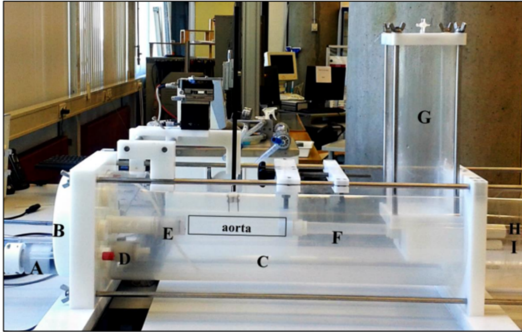
Figure 2.6: Experimental setup for the extension-inflation test [64].
