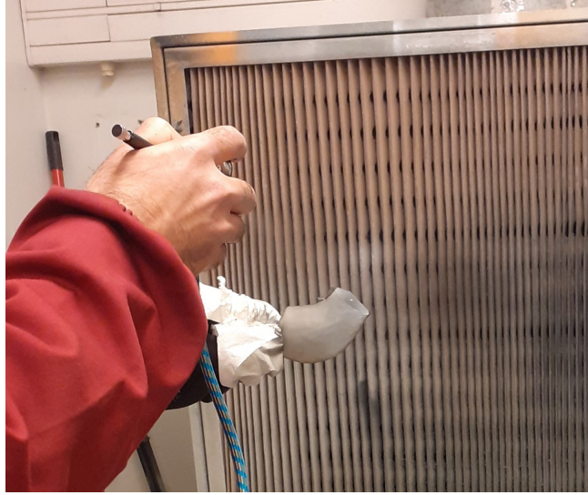
Figure 4.3: Attempt to create a speckle pattern with Titanlux paint.
