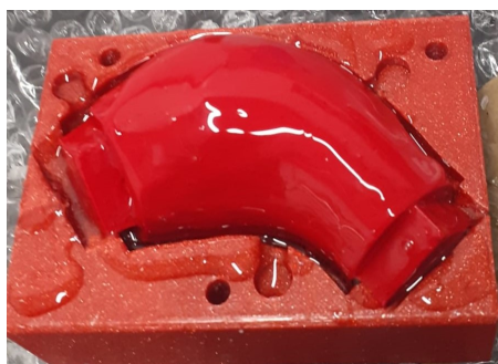
Figure 3.16: Liquidity of the Sylgard 184 mixture in the mold.
