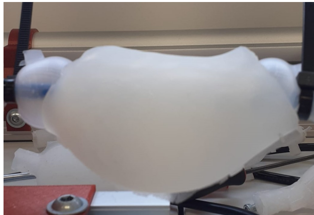
Figure 3.21: Dislodgement of the balloon from the phantom at a pressure below 120 mmHg.
