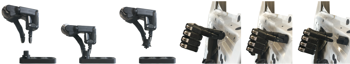
Figure 6.13: Wiring fitting task: steps 1 to 6, from left to right, respectively
