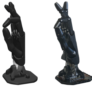
Figure 5.4: Hand pose replication in simulation (left) and in reality (right) by BioIK before taking into account the joints coupling
