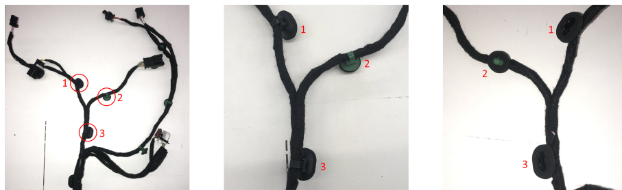
Figure 5.7: Clips utilised for the wiring fitting task
