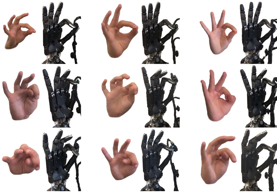
Figure 5.30: Successful grasps from tests. The rows, from top to bottom, correspond to the DexPilot, BioIK and TeachNET algorithms, respectively. The left to right columns correspond to clips 1, 2 and 3, respectively.
