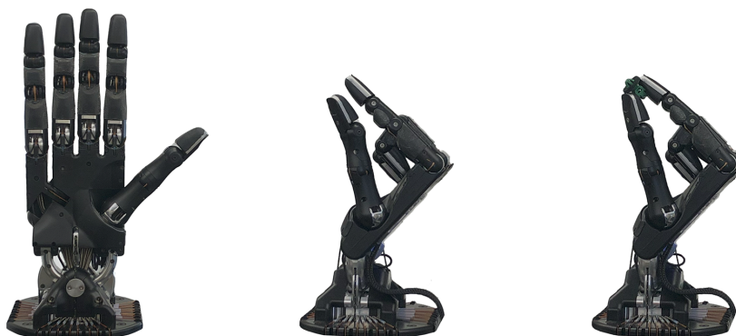
Figure 6.4: Hand Positions for states "Hand_Open", "Start_Pinching_Position" and "Pinching_Position", respectively
