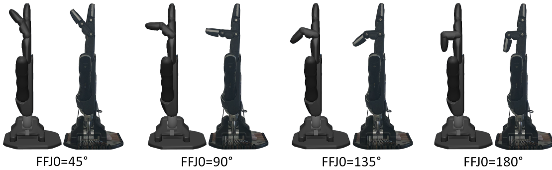
Figure 5.6: Joints coupling test qualitative results in MuJoCo and in the real Shadow Hand
