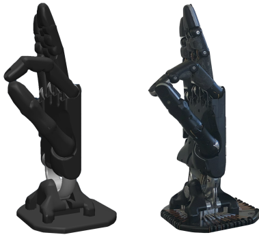
Figure 5.2: Hand pose replication in simulation (left) and in reality (right) by DexPilot before taking into account the joints coupling
