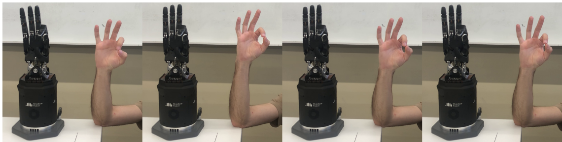
Figure 5.10: DexPilot: pinching pose repeatability
