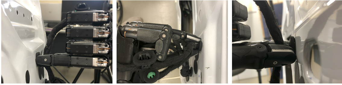
Figure 6.5: Unsuccessful clipping attempt with the developed algorithm (left, top and right view-points, respectively)
