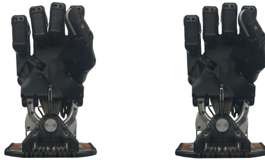
Figure 6.6: Clenched fist hand positions for states “Start_Pinching_Position” and “Pinching_Position”, respectively
