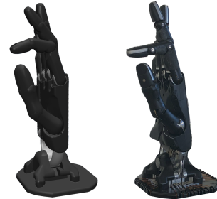
Figure 5.5: Hand pose replication in simulation (left) and in reality (right) by BioIK after taking into account the joints coupling
