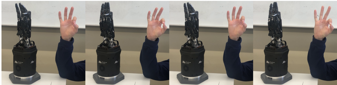
Figure 5.13: BioIK: pinching pose repeatability
