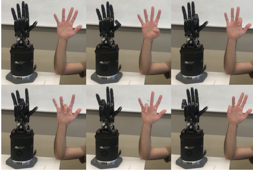
Figure 5.8: Direct joints mapping algorithm test results
