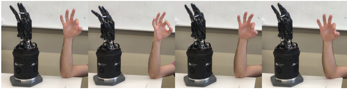
Figure 5.18: TeachNET: pinching pose repeatability
