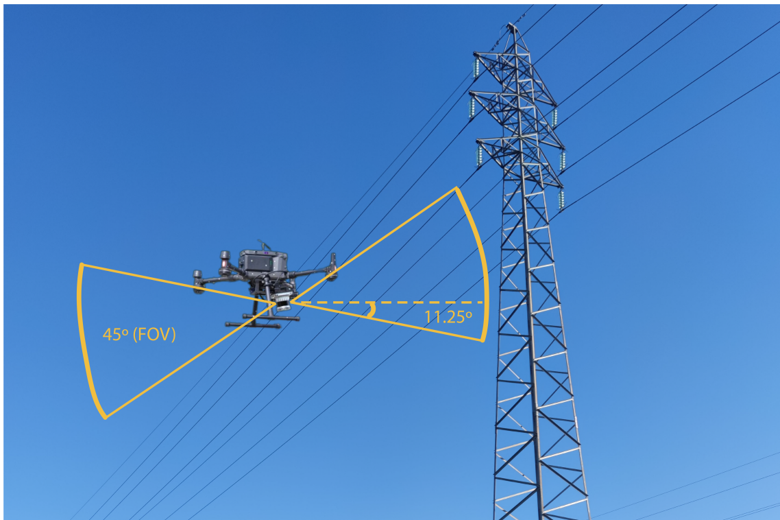
Figure 5.3: Inclination of the LiDAR on the drone
