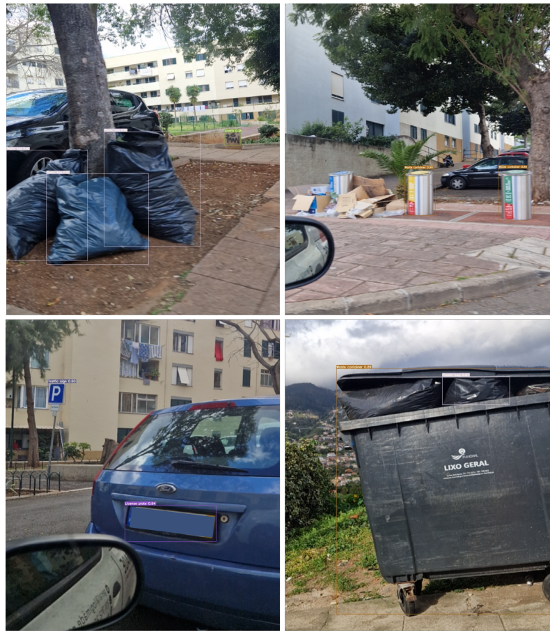
Figure 5.13: Testing images annotated using training 5 in table 5.9 (white bounding boxes for "plastic bag", green for "graffiti", brown for "waste container", grey for "traffic sign, and purple for "license plate")
