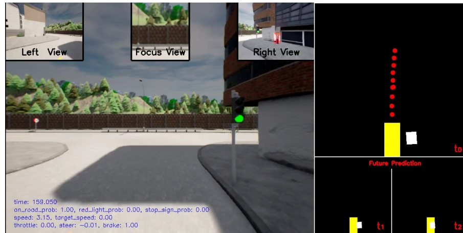
Figure 5.7: InterFuser Algorithm Mistake Due To Big Shadow.
