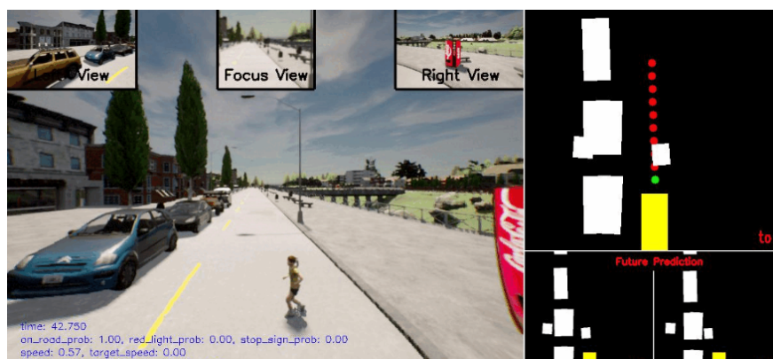
Figure 3.4: Algorithm's Views and Sensors.
