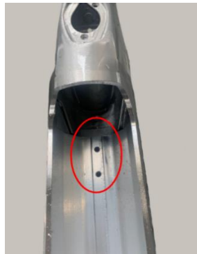
Figure 41 - Two of the six holes to be drilled on the DT.
