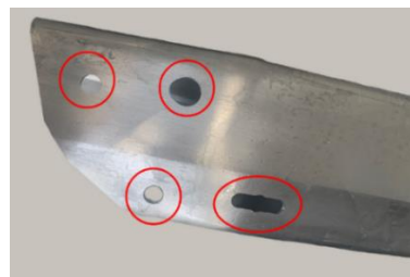
Figure 34 - Machined slots and holes on the DT on Model #2.
