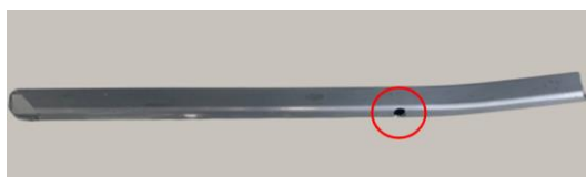
Figure 35 - Machined hole for the SS on Model #1.
