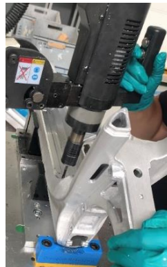
Figure 18 – Manual threading of the holes on the frame part (operation 7).
