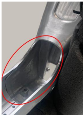
Figure 37 - Machining of the top of the DT's surface.
