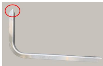
Figure 29 - Machining of the SS to fit the ST on Model #2.
