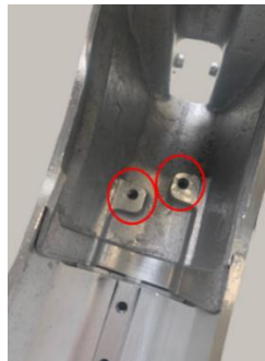
Figure 38 - Machining of the slots on the DT.
