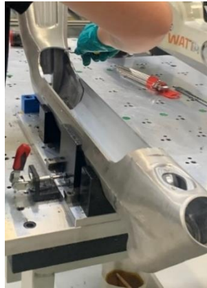
Figure 19 – Manual deburring of the frame part (operation 6).
