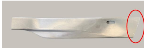
Figure 32 - Machining of the CS to fit the MB on Model #2.
