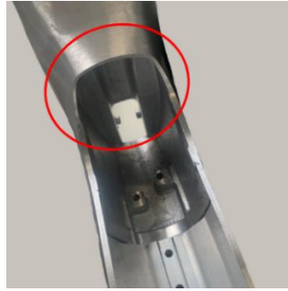
Figure 39 - Widening of the access to the battery on the DT.
