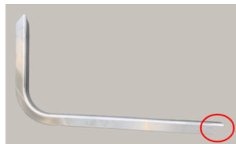
Figure 30 - Machining of the SS to fit the Dropouts on Model #2.
