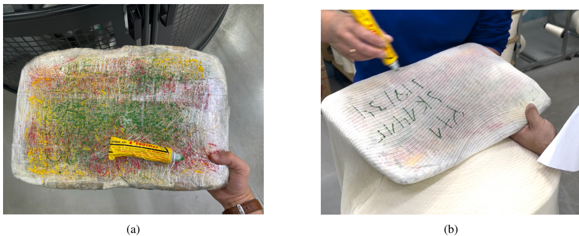
Figure 4.1: Standard method for marking rolls. (a) The material used (b) A roll being marked for further identification
