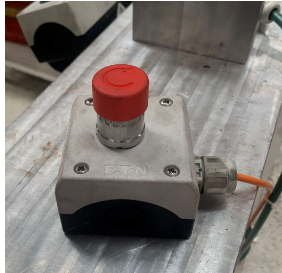
Figure 3.41: Emergency button control box.
