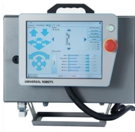
Figure 3.2: CB3 teach pendant and control box [5].
