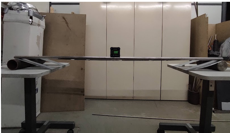
Figure 4.8: Measuring inclination with respect to both supports
