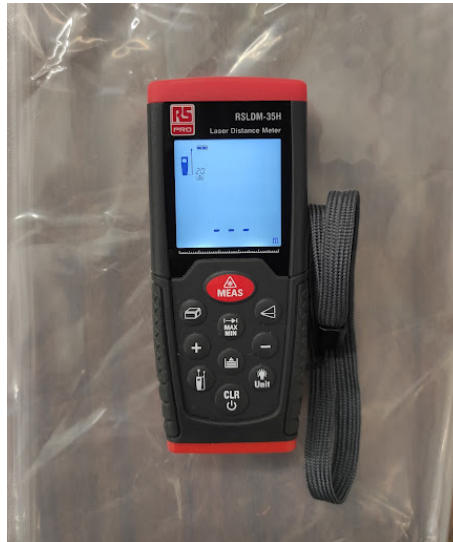
Figure 4.7: Laser distance meter used
