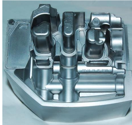
Figure 37- CrN coated (Titanit).
