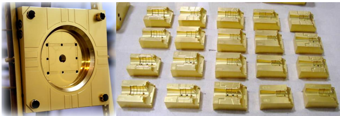
Figure 36- TiN coated mold cavity (Surface Solutions Inc.).
