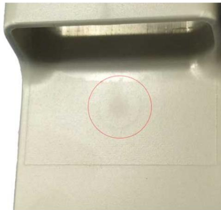
Figure 27- Blush defect, (Boyanmfg, 2020).
