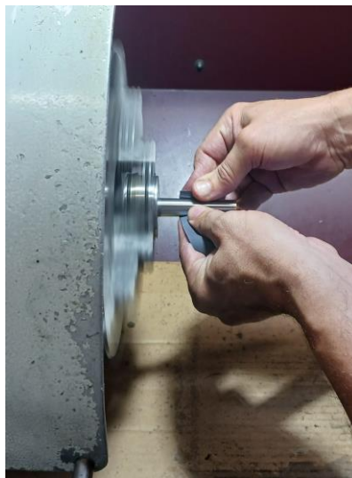
Figure 68- Un-polishing the bush on a conventional lathe machine, manual work.
