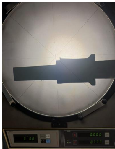
Figure 53- Dimensional inspection on a profile projector.
