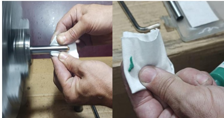
Figure 69-Polishing the bush with diamond past.
