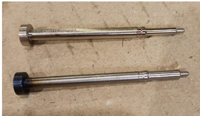
Figure 44- Muroplás pins, before (down) and after (up) the treatment.
