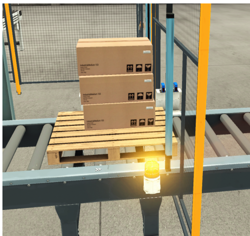
(a) Muting active and muting enable command inactive
