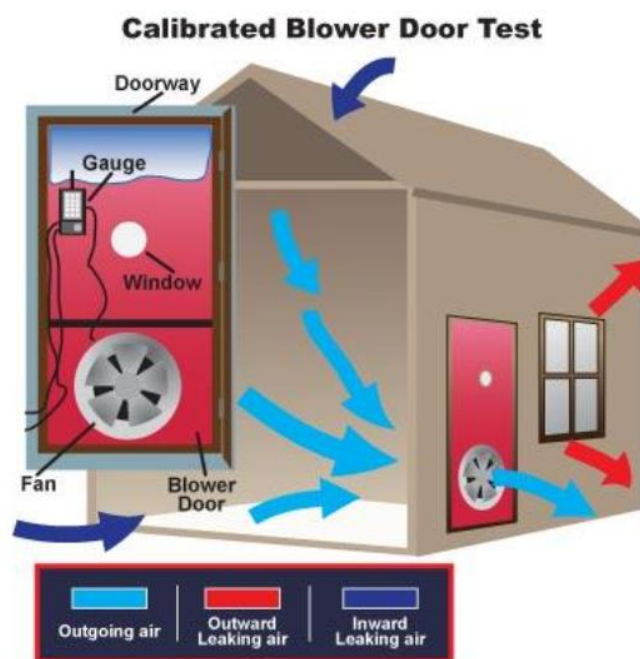
Figura 3.9 – Blower Door Test [57]
