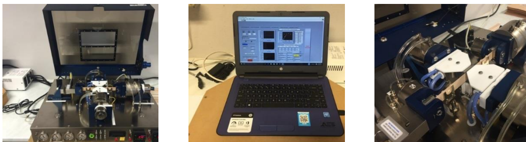
Figura 4.16 – ABES (Automated Bonding Evaluation System)
